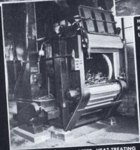
CLEANING KEN-TOOLS AFTER HEAT-TREATING OPERATION
